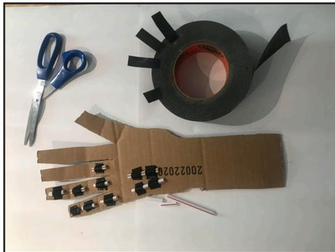
**3. Add Tendon Sheaths:** Cut a straw into small lengths that can fit between the finger joints. Cut a longer piece of straw for each finger in the palm of the hand. Tape or hot glue the straw pieces down.
